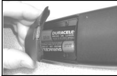
Figure 1- 9 Re-inserting the battery door
