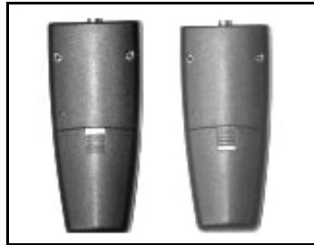
Figure 1- 7 Moving the battery door sliding tab
